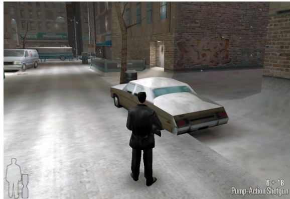
FIGURE 3: Ordered grid 4x multi-sampling in Max Payne. The impact of using less texture data becomes very apparent. The sign that appears to be clear above is now blurred.
