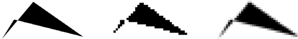
Figure 4: A shape (left) resampled from 512 \times 512 to 100 \times 100 pixels in Photoshop, using nearest neighbor (i.e. not filtered, middle) and bicubic (right) filtering. Notice the jagged edges, and detail breaking up in the thinner portion in the middle image.
