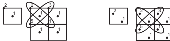
Figure 11: NVIDIA Quincunx™ sample points (left) and shifted points of Accuvie™ (right).
